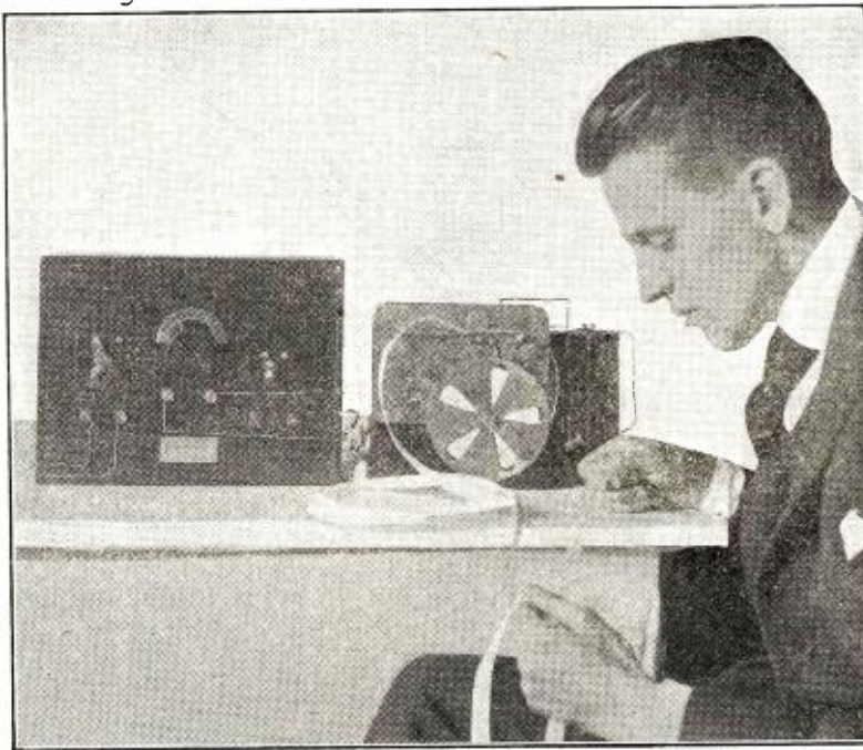
William G. H. Finch, the Inventor of the Radio Signal Recorder. The Illustration Also Shows the Essential Instruments Connected With the Successful Operation of the Device. It is Claimed for This Invention That it Will Accurately Register on Tape Radio Signals up to 2600 Miles When Employing a Vacuum Tube Receiver Circuit.
